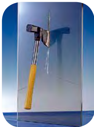
Security glass test using an axe Classes: P6B, P7B, P8B
